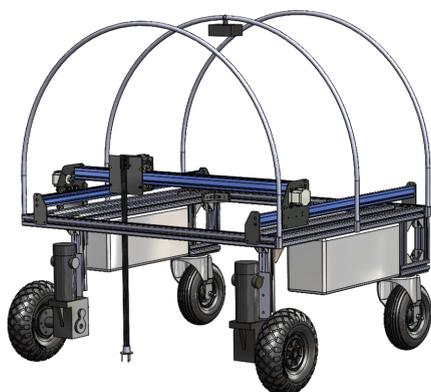
Scenario 1 already covers the use of the robot for weeding but there is a need to test the weeding robot without a cablebot, database server or weeding map. Scenario 3 is therefore a more “conventional” scenario in which the robot navigates autonomously and combines 1) the use of classical, mechanical weeding tools in between the rows of plants and 2) the CNC arm to weed in between the plants on a row.
