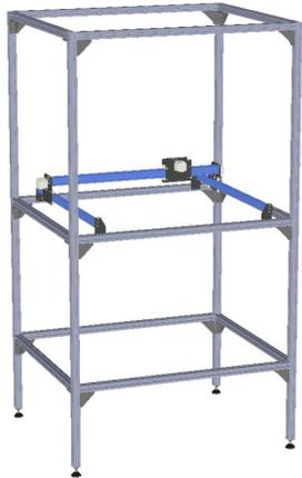
The scanner is our development environment for the 3D scanning algorithms. The installation is an accessible (meaning: not too expensive) solution for plant phenotyping that may be useful for research labs.
